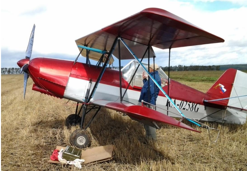
Figure 1: The plane "Shmel'" that operating on the conversion engine Subaru EJ-25 which used for research.
