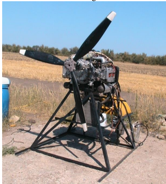
Figure 2: Test bench for testing the performance of engines applied in aviation.
