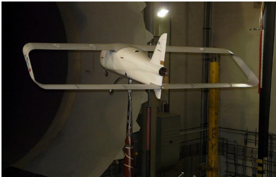
Inverted Joined Wing Airplane Flying Model tested in the wind tunnel of the Institute of Aviation
