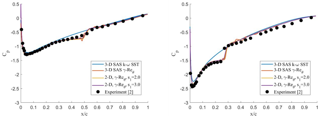
Figure 3 – Pressure coefficient distributions  $C_p$  along the NACA 0018 airfoil surface for angles of attack  $AoA=4deg$  (left) and  $AoA=8deg$  (right).
