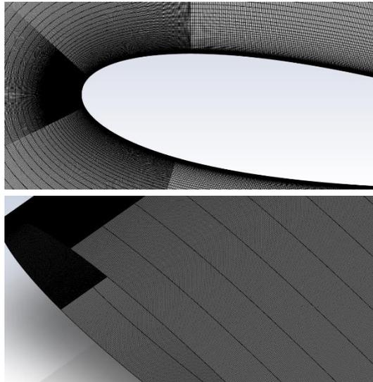
Figure 2 – Mesh around the NACA 0018 airfoil. The top view shows the structured mesh near the airfoil surface, focusing on the boundary layer, while the bottom view highlights the uniform spanwise cell distribution for 3-D simulations.
