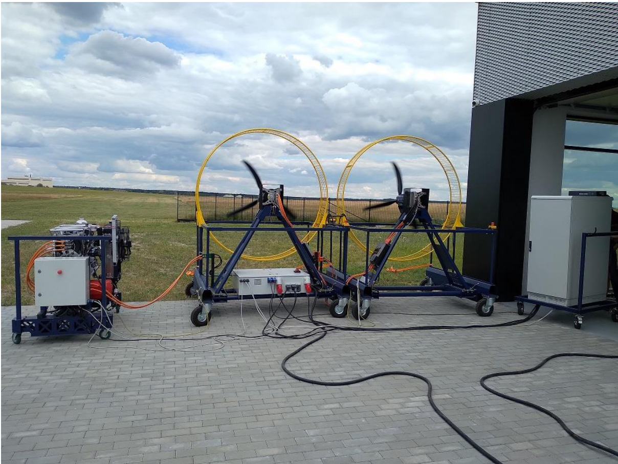
Fig. 2 The ground testbed of the propulsion system.
