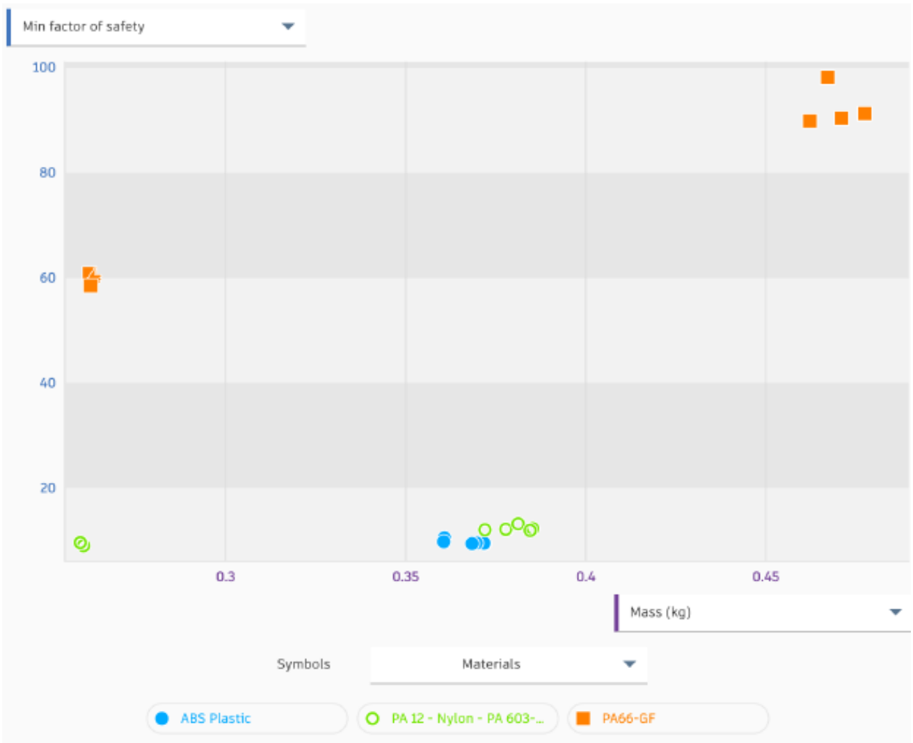
Figure 15 - The output geometries are presented on the plot, showing their mass and corresponding safety factor
