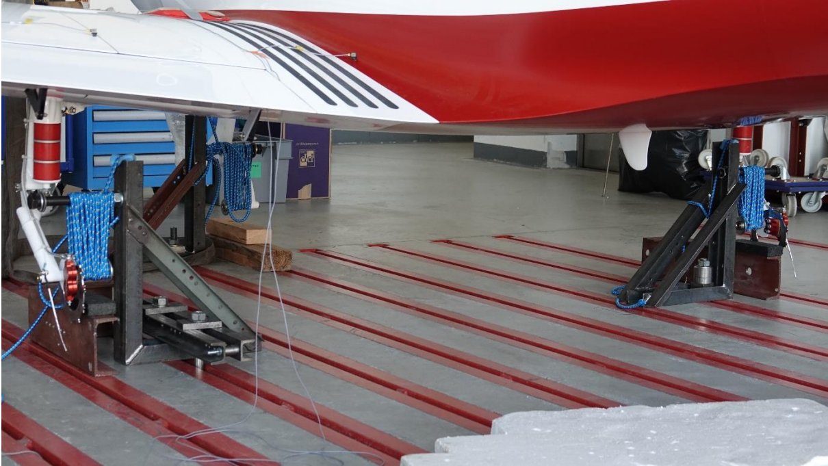
Figure 1 - The aircraft suspension during the ground vibration testing
