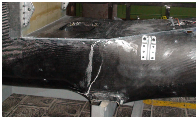
Figure 2: Damage area of VUT 061 Turbo fuselage.
