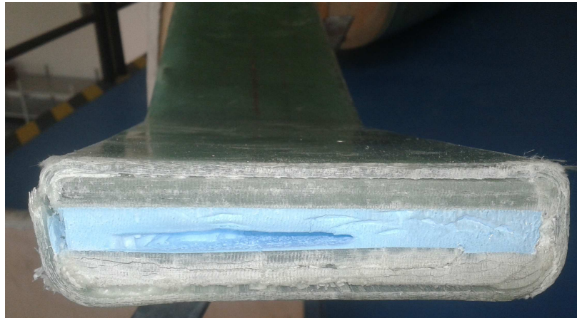
Figure 1: Landing gear core crushing.
