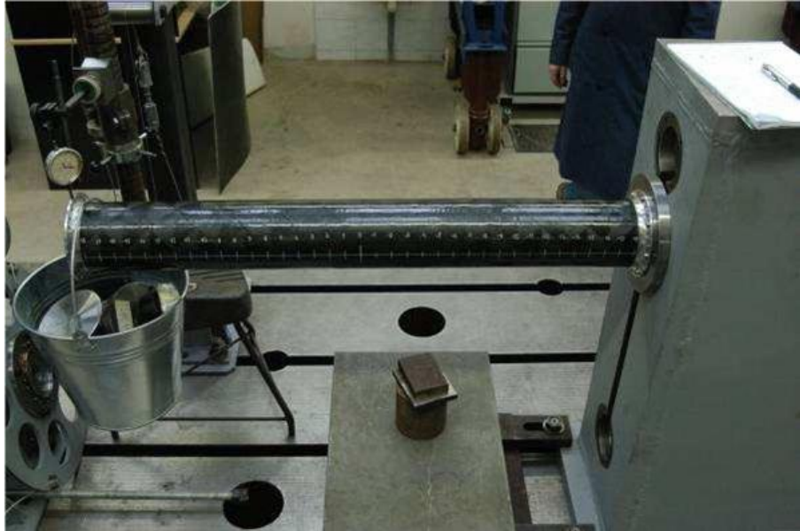
Figure 4: The transmission shaft undergoing bending stiffness test [4]
