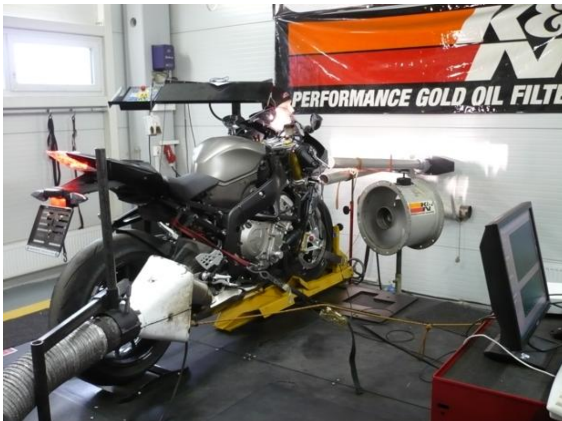
Figure 9: The BMW S1000RR motorcycle during cylinder pressure measurement [2]
