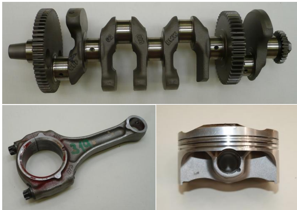
Figure 7: The components of the crank mechanism of the BMW S1000RR engine [2]
