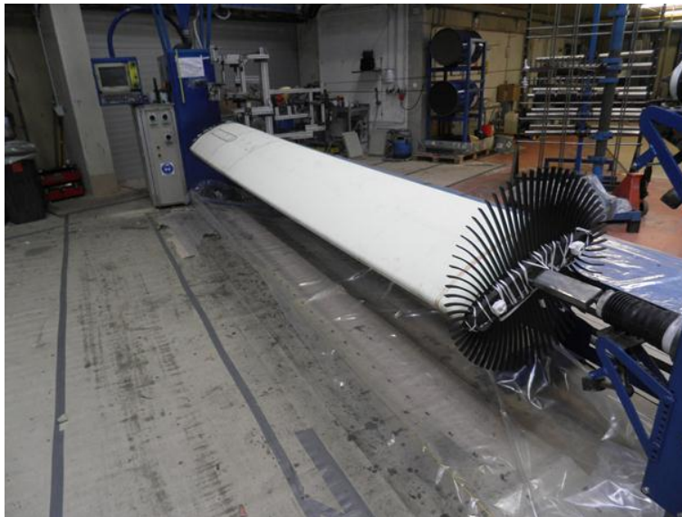
Figure 12: Winding machine and wing segment.
