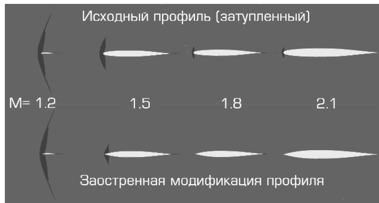
Figure 6: Local subsonic zones for different M numbers for blunt (top) and sharp (bottom) airfoils
