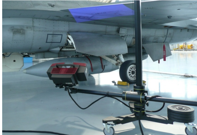
Fig. 4 ATOS II Triple Scan in use – scanning points on wing lower skin.
