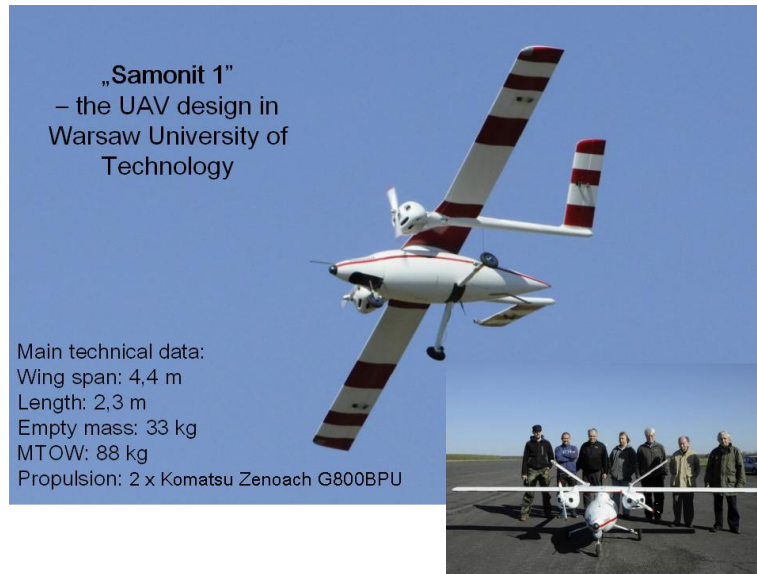
Fig. 1 SAMONIT 1 – the UAV and its technical data
