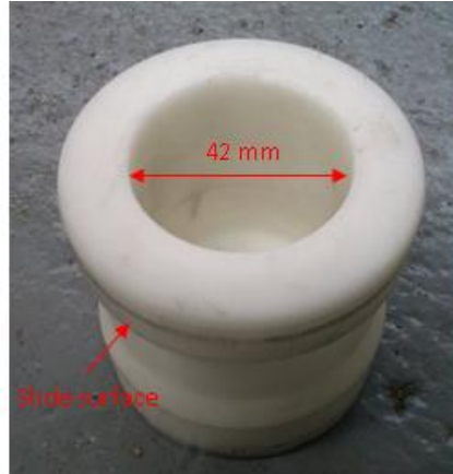
Figure 2 Sabot used for simulated hailstone impact testing.
