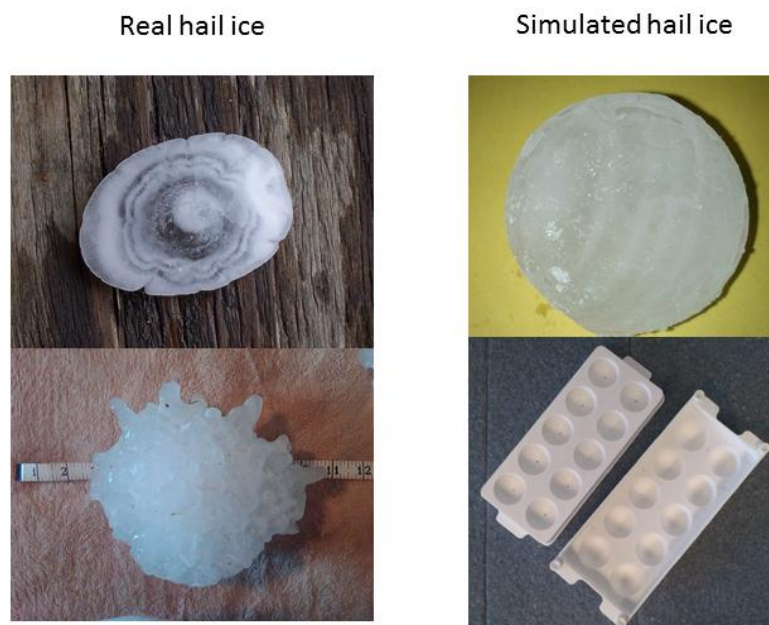
Figure 4 Real and simulated hailstone comparison.
