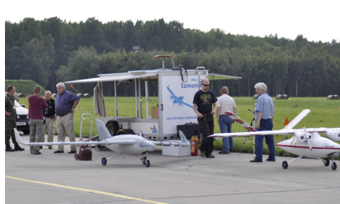
Fig. 7 Ground preparation for flight-testing. Tailless, pushing propeller airplane on the left, the classical V-tail configuration on the right and Ground Control Station (also used for transport of airplane parts) behind. Minsk Mazowiecki, July 2011.
