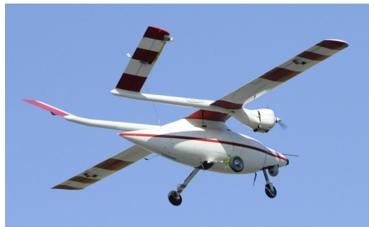
Fig. 5 Airplane in tailed, tractor configuration. Flight test with autopilot in the loop. Daylight camera (FLIR) visible at the nose of the container. Sochaczew, April 2011.
